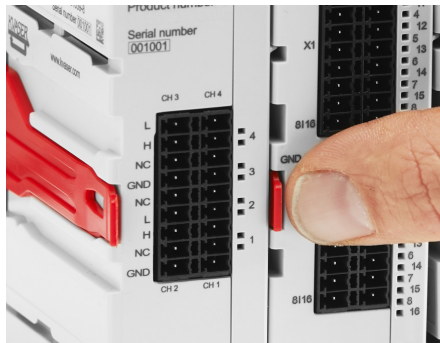
Figure 6: Press the top of mounting clip before removing a module from the DIN Rail.
